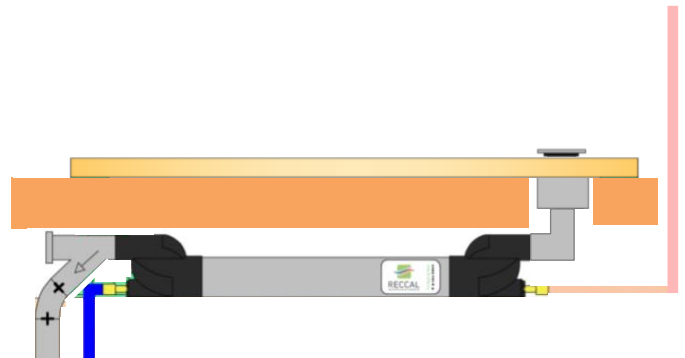
Unsecured positioning of the receiver
